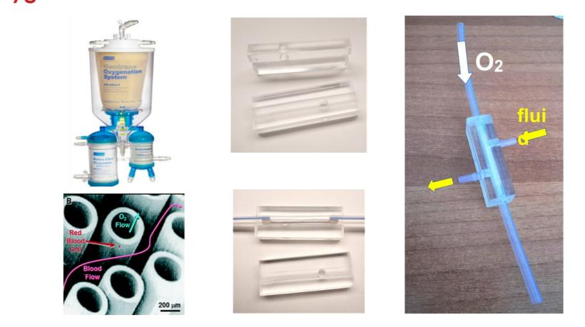
The mini-oxygenator is based on **hollow fibers** derived from a discharged oxygenator system. The housing consists of two drilled Plexiglas blocks sealed with two-component adhesive and containing the hollow fibers. The **oxygen flows** through the fibers, while the perfusate around them.
